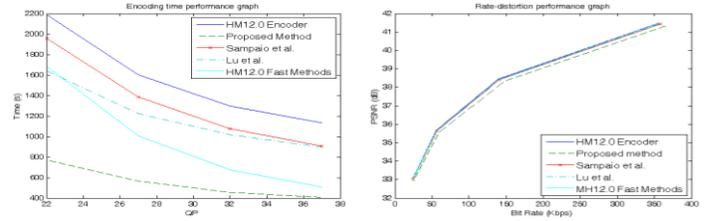
Fig. 2. Encoding time and RD performance for the ‘Container’ sequence.
