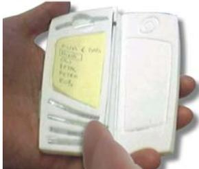
**Figure 1** "Soft" model with replaceable Post-It note screens
