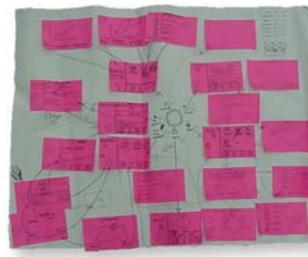
**Figure 4.** *Post-It* State Transition Diagram
