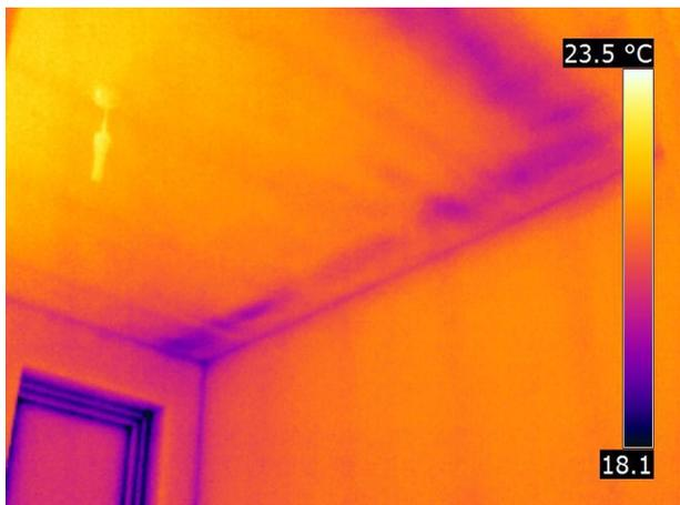
(a) The reduced surface temperatures along the ceiling follow a linear pattern corresponding with the position of the MVHR unit ductwork
