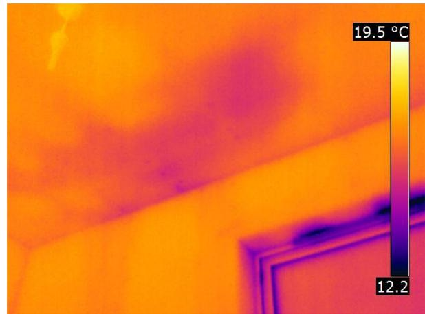
(b) Thermal image shows localised surface temperature decrease in ceiling area corresponding with the position of the extract duct for the mechanical ventilation unit
