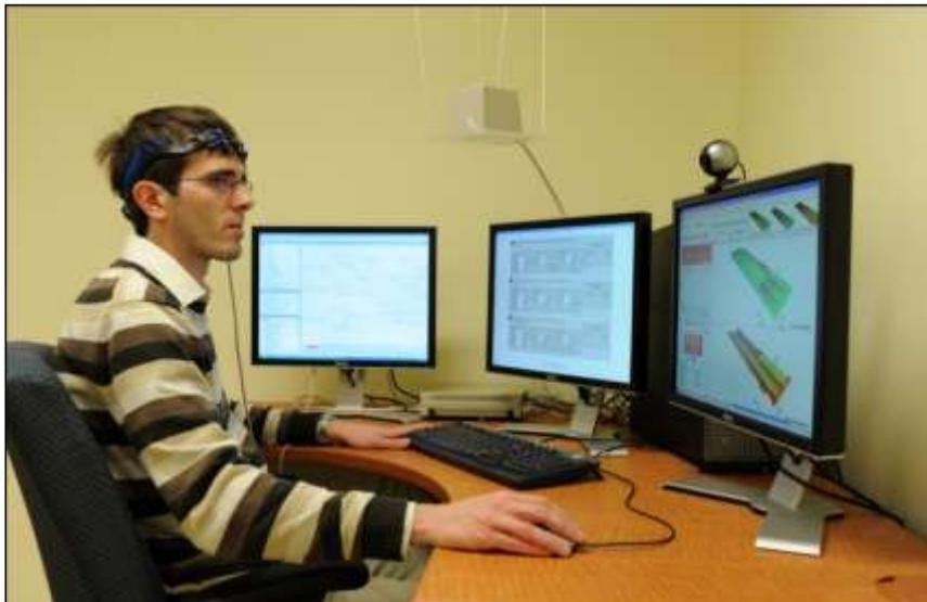
Figure 4. Experimental setup in the IMAGE-Desktop condition. The screens were disposed in an arc in front of the participant. Each screen was assigned to a specific function, namely knowledge representation (left), interactive simulation (center) and enhanced visualization (right). Although not described in the present article, participants were required to wear a head-tracking device which was used for behavioural measurement and design recommendations.
